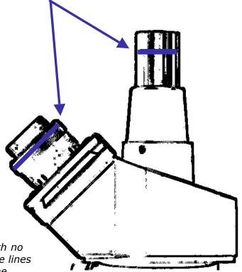
A basic trinocular head with no eyepieces inserted. The blue lines indicate the location of the intermediate image. The image in the trinocular tube must somehow be placed on the camera sensor. There are several ways of accomplishing this. But first there are some important factors that must be considered for best results.
